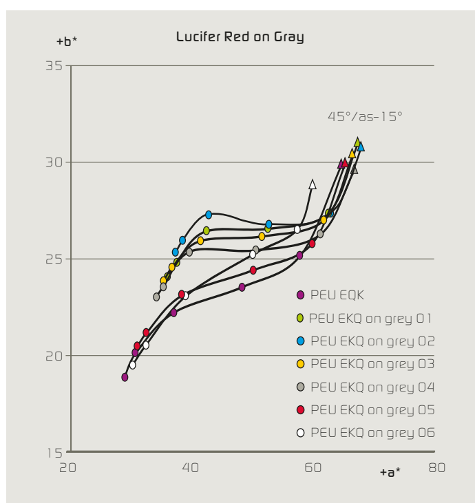
Figure 5: The colour lines (aspecular lines) in the sample deviate from the reference sample over the grey graduations, especially at large aspecular angles. Colour values are summarised here as lines from 45°/as110° (left) to 45°/as-15° (at right).
